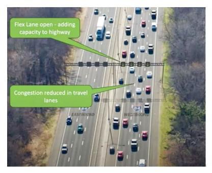
A rendering of how the inside shoulder of I-84 in Danbury could be opened to reduce rush hour congestion. Note that on the right, heavy westbound traffic is using the shoulder. On the left, since traffic is lighter, the shoulder is closed.
