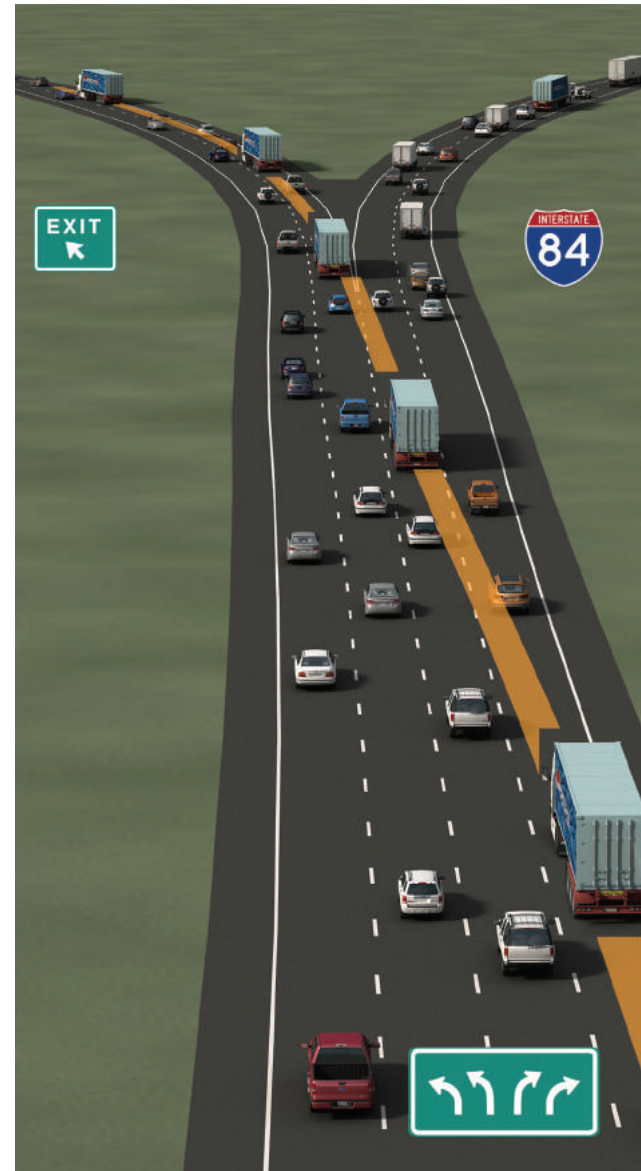
Ramps on the left mean traffic must cross lanes to exit
