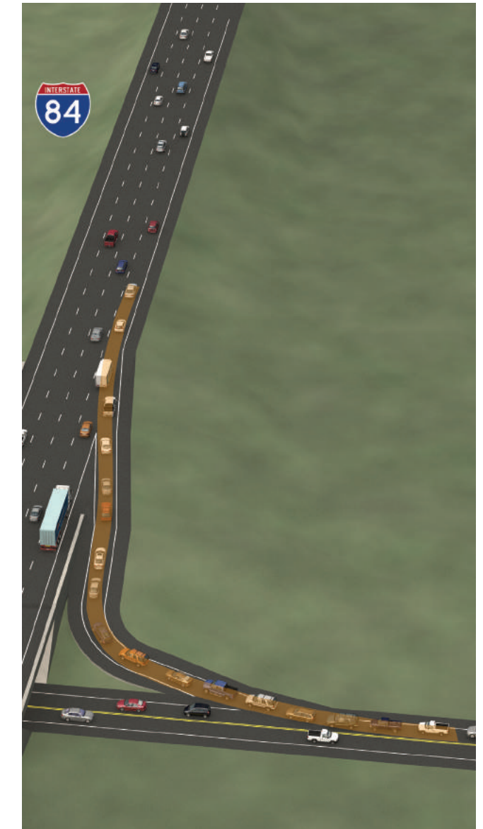
Short ramp lengths cause traffic backups
